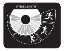
The STRIDE LENGTH display presents a visual representation of the length of your stride. The lighted pendulum swings to the right as you stride forward with your right leg and swings to the left as your left leg moves forward.
